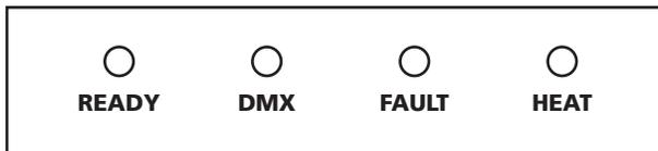
**READY:** Flashing means heating up, about 5min. Turns from flashing into long on, indicates that the machine is ready to work.
