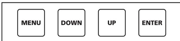
**MENU:** switch through setup menu. Press 3s switch to advanced interface
